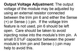
With a resistor between the trim pin and Sense (-) pin, the output voltage is adjusted down. To adjust the output voltage down a percentage of Vout ( $\Delta$ %) from Vo,nom, the trim resistor should be chosen according to the following equation:
